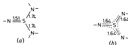
Fig. 5. Two characteristic arrangements of S—N lengths for a trigonal pyramidal S(IV)N 3 moiety as found in (a) 1-phenylimino-2,5-diphenyl-1 \lambda^4 ,2,5-thiadiazolidine-3,4-dione (Neidlein et al. , 1977) and (b) K 2 [S(NTs) 3 ] (Gieren & Narayanan, 1975).
